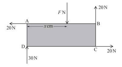
An additional force FN is also applied at right angles to AB to a point on the edge AB x cm from A.
