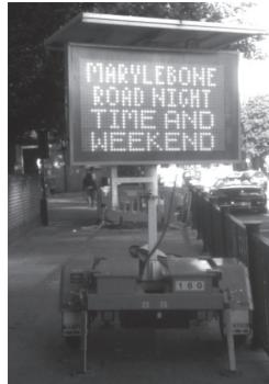
The traffic sign uses many small lights all powered by a rechargeable battery. These lights need to be very bright during the day so that they can be seen clearly. They do not need to be as bright at night.
