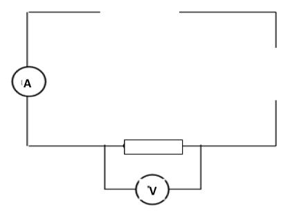
(i) The diagram needs a switch and a single cell or battery.
