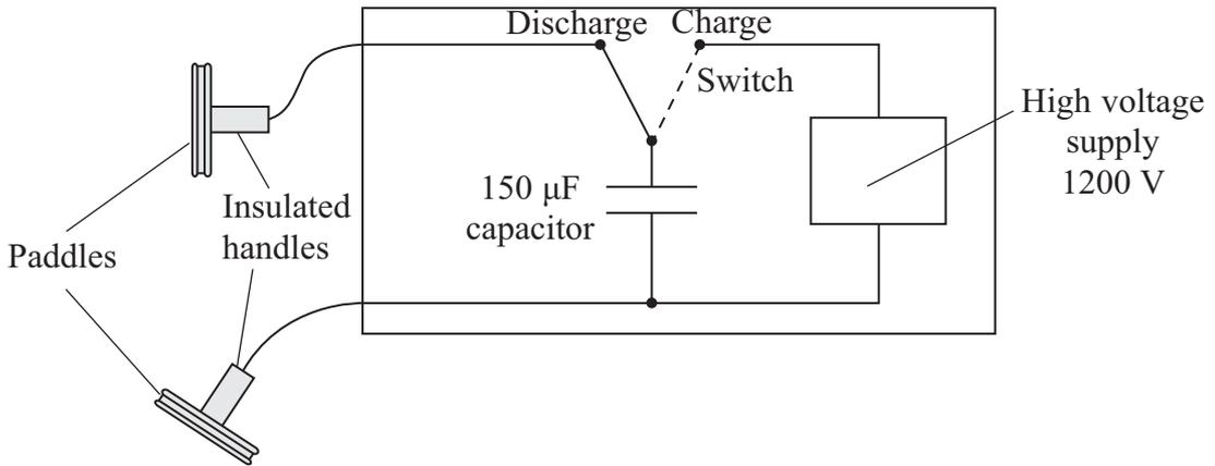
(a) The  $150 \mu\text{F}$  capacitor is first connected across the  $1200 \text{ V}$  supply.
