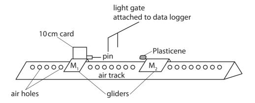
The student pushes the first glider M<sub>1</sub> towards glider M<sub>2</sub>, which is stationary.
