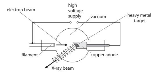
(i) The electrons in the beam escape from a hot filament.
