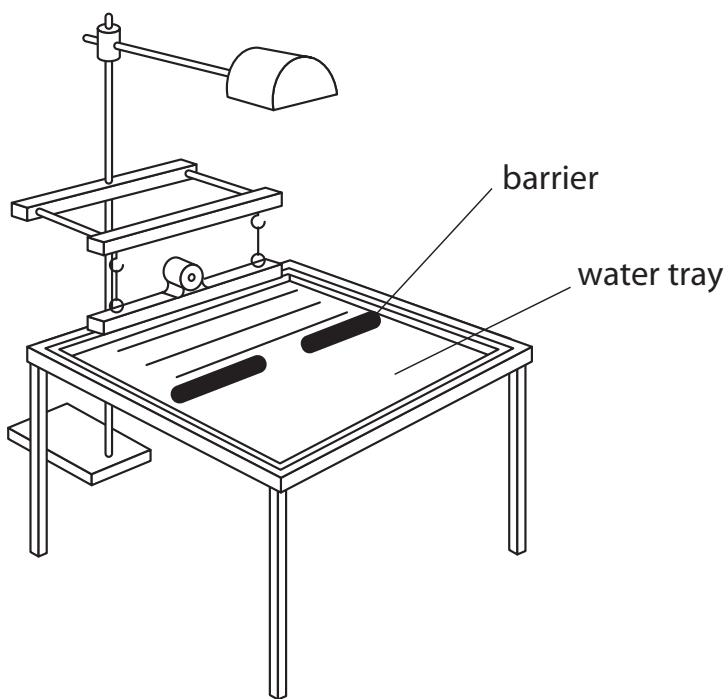
The ripple tank produces plane waves.
