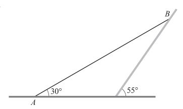
A uniform rod AB, of weight 20 N and length 2.8 m, rests in equilibrium with the end A in contact with rough horizontal ground and the end B resting against a smooth wall inclined at 55° to the horizontal. The rod, which rests in a vertical plane that is perpendicular to the wall, is inclined at 30° to the horizontal (see diagram).
