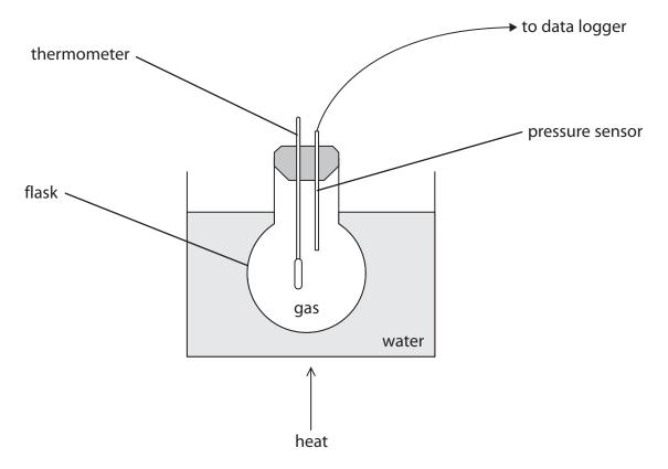
(a) The volume of the gas is kept constant by the flask.
