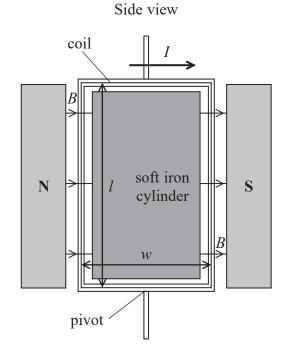
The fixed soft iron cylinder and magnets produce a uniform magnetic field of magnetic flux density B. The coil is able to rotate within this magnetic field. The coil has width w and length l. There is a current l in the coil in the direction shown in the side view diagram.
