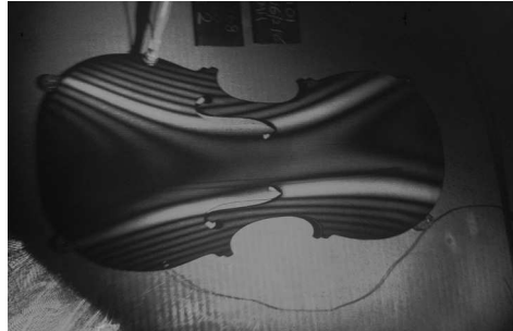
Fig. 5: Chladni standing wave pattern on a vibrating violin plate imaged using holographic techniques
