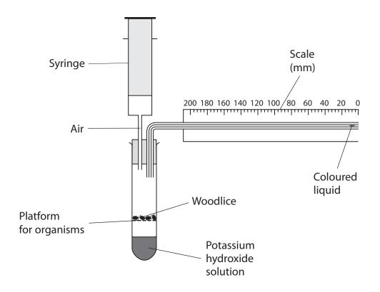
(a) (i) Potassium hydroxide solution absorbs carbon dioxide. Suggest a reason for absorbing carbon dioxide in this apparatus.
