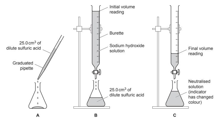
The student adds sodium hydroxide solution from the burette to the sulfuric acid until the indicator changes colour.
