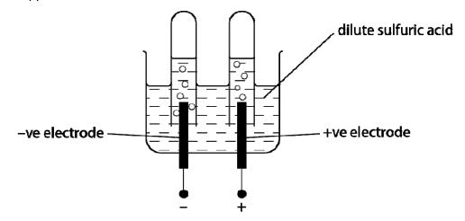
Hydrogen is made at the negative electrode.
