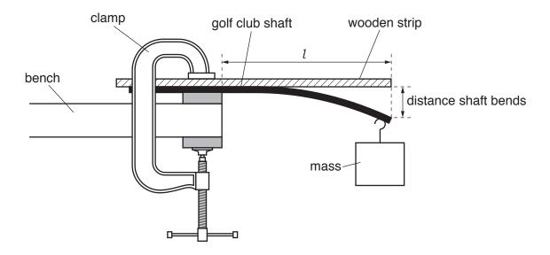
He measures the distance that the shaft bends when the mass is added.
