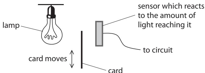
The piece of card can be moved up and down between the lamp and the detector. Each part of the teacher's arrangement corresponds to a part of the machine.
