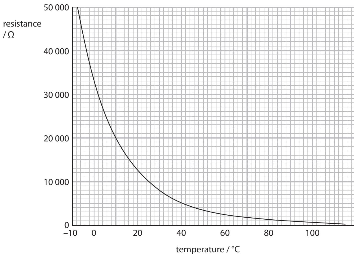
When the temperature is  $10^{\circ}\text{C}$ , the current in the thermistor is 0.60 mA.
