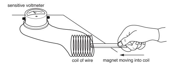
When Alyssia pushes the magnet into the coil the voltmeter reads 2 mV.
