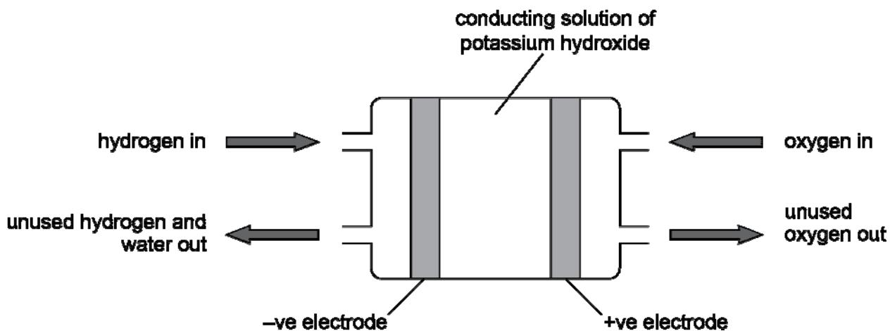
Potassium hydroxide solution contains potassium ions,  $K^+$ , and hydroxide ions,  $OH^-$ . Water,  $H_2O$ , is made in this type of fuel cell.
