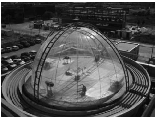
A 'smog chamber' at the European Photoreactor (EUPHORE) in Valencia, Spain
