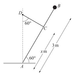
A uniform rod AB of mass 4 kg and length 3 m rests in a vertical plane with A on rough horizontal ground.
