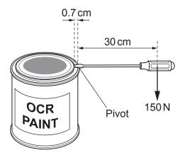
What is the clockwise moment of the screwdriver about the pivot? Use the Data Sheet.
