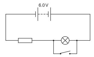
The lamp and the resistor each have a resistance of  $5.0\,\Omega$  so that the total resistance in the circuit is  $10.0\,\Omega$ .
