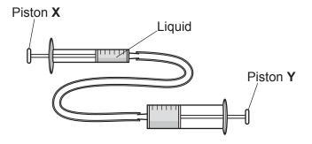
Piston **X** is pressed with a force of 10 N. What is the force produced at piston **Y**?
