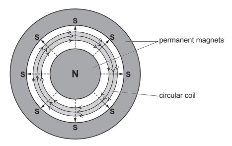
The magnetic field through the coil has strength 0.40 T.
