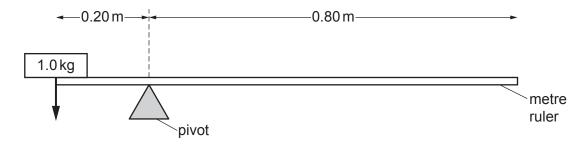
(a) Calculate the moment of the 1.0 kg mass about the pivot, in units of Nm.
