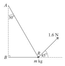
A light inextensible string has its ends attached to two fixed points A and B. The point A is vertically above B. A smooth ring R of mass m kg is threaded on the string and is pulled by a force of magnitude  $1.6\,\mathrm{N}$  acting upwards at  $45^\circ$  to the horizontal. The section AR of the string makes an angle of  $30^\circ$  with the downward vertical and the section BR is horizontal (see diagram). The ring is in equilibrium with the string taut.
