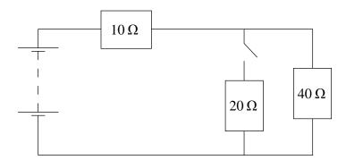
When the switch is closed, the potential difference across the  $20 \Omega$  resistor would
