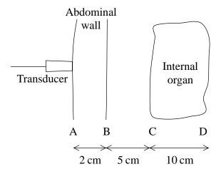
(i) Calculate the time interval between sending out a single pulse and receiving its echo from interface B. The speed of ultrasound in the abdominal wall is  $1500\,\mathrm{m\,s^{-1}}$ .
