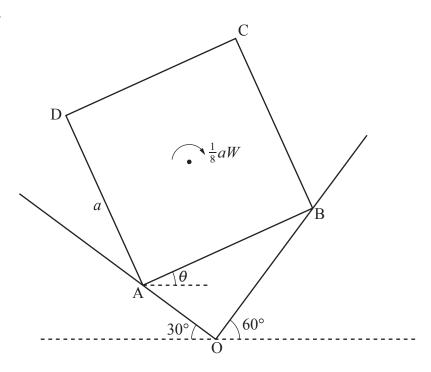
The diagram shows a uniform square lamina ABCD, of weight W and side-length a. The lamina is in equilibrium in a vertical plane that also contains the point O. The vertex A rests on a smooth plane inclined at an angle of  $30^{\circ}$  to the horizontal. The vertex B rests on a smooth plane inclined at an angle of  $60^{\circ}$  to the horizontal.
