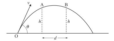
A particle is projected with speed v from a point O on horizontal ground. The angle of projection is  $\theta$  above the horizontal. The particle passes, in succession, through two points A and B, each at a height h above the ground and a distance d apart, as shown in the diagram.
