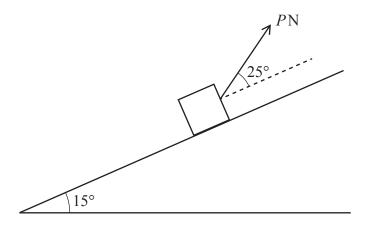
The pulling force has constant magnitude PN and acts at a constant angle of 25° above the slope, as shown in the diagram.
