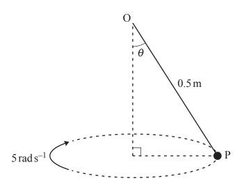
The diagram shows a particle P, of mass 0.1 kg, which is attached by a light inextensible string of length 0.5 m to a fixed point O.
