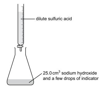
The equation for the reaction is shown.
