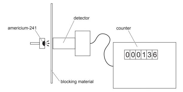
They recorded the number of counts detected in one minute with different blocking materials.
