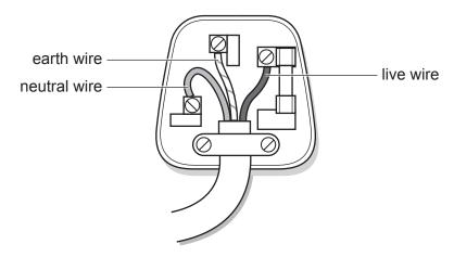
(a) (i) Put a tick (✓) in the correct box in each row to show the correct descriptions of the live, neutral and earth wires.
