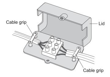
The cable grips are important parts of the connecting box.
