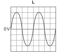
In each diagram, one vertical division on the oscilloscope screen represents 2 volts.
